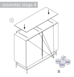
Position the silicone suckers in the grooves on top of the carcass and then rest the glass top in place.
