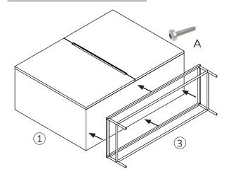
Attach the Wide Base (Carton 3) to the **2 x two-door carcasses** (Carton 1). Place the carcass on its back and fix using the self tapping screws 'A'. There are pilot holes to align the base. Once the bases has been secured **(with minimum 2 x people)** you will need to lift the sideboard off its back and onto the base. **DO NOT PIVOT ON ONE BASE LEG.**
