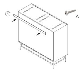
Fix the wide back plate (Carton 4). With a screwdriver attach the backplate by aligning with the pilot holes and using the self tapping screws 'A'.
