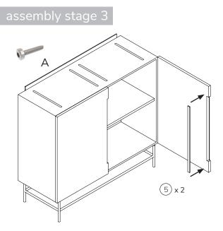
Attach the finger plates to the rear of both doors using the self tapping screws provided.
