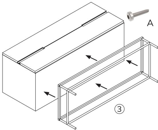
Attach the Wide Bases (Carton 3) to the **drawer & door carcasses** (Cartons 1). Place the carcasses on their backs and fix using the self tapping screws 'A'. There are pilot holes to align the bases. Once the bases has been secured (**with minimum 2 x people**) you will need to lift them off their backs and into an upright position. **BE CAREFUL NOT TO REST / PIVOT ON ONE BASE LEG.**
