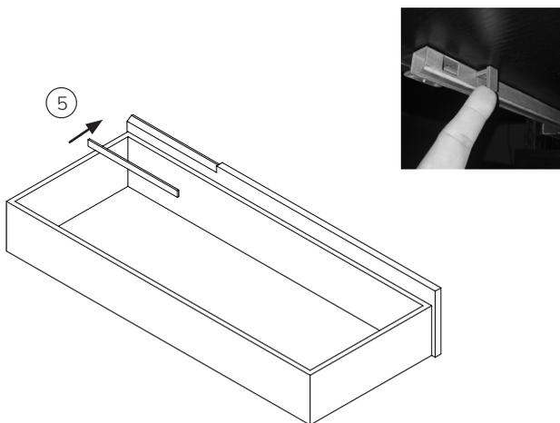
Attach the small finger plates '5' using the self tapping screws provided. It may be easier to remove the top drawers (not essential) and this can be done by releasing the drawer from the runners - see photo above.
