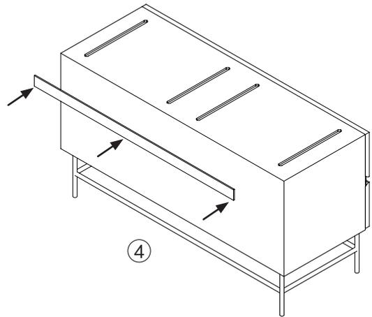
Fix the long back plate (4) to the rear of each carcass using a screwdriver and the self tapping screws and align to the pilot holes.
