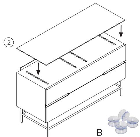
The final stage of the assembly is to place and position the glass tops. Place the silicone suckers 'B' into the grooves on top of the carcasses and then rest the glass tops '2' in place.
