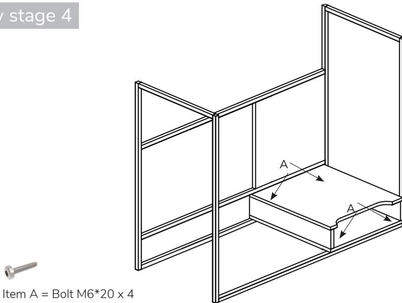
Attach the drawer carcass to the frame using 4 x screw (A). NB. Make sure the carcass is the correct way up (pre-drilled bolt holes facing the frame). Once fixed in place 'press the back panel into its original position and securely engage the drawer back onto its runners'
