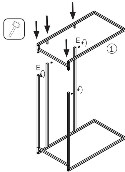
Place the second side frame in position and gently tap onto the rails ensuring the parts are tightly together before securing with the screws (E)
