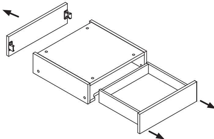
Release and remove the drawer by pressing (in opposite directions) the small plastic lever on each runner and then gently press the back panel from inside the carcass.
