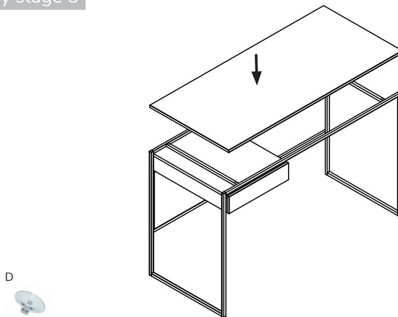
Place plastic suckers into frame holes and gently lower glass into place.
