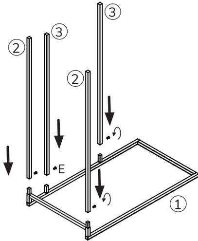
Place one side frame (1) on the floor and insert the rails as shown securing with the screws (E)
