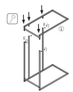
Place the second side frame in position and gently tap onto the rails ensuring the parts are tightly together before securing with the screws (E)
