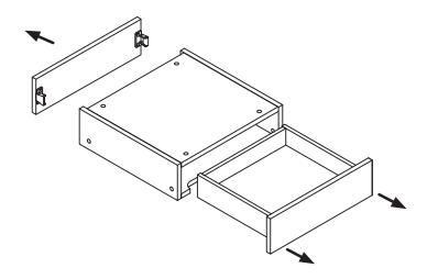
Release and remove the drawer by pressing (in opposite directions) the small plastic lever on each runner and then gently press the back panel from inside the carcass.
