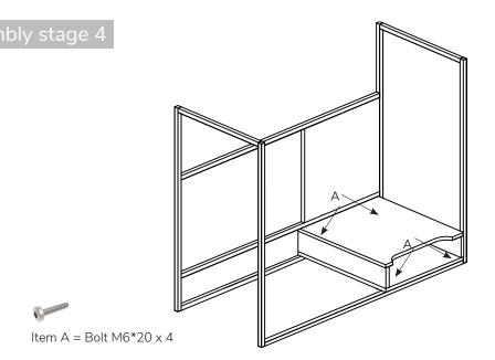
Attach the drawer carcass to the frame using  $4 \times \text{screw (A)}$ . NB. Make sure the carcass is the correct way up (pre-drilled bolt holes facing the frame). Once fixed in place 'press the back panel into its original position and securely engage the drawer back onto its runners'
