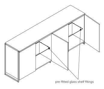
place and fix glass in place with supports pre-fitted to the carcass interior.
