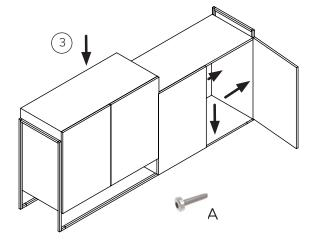
with the frame upside down, place the Carcasses (carton 4) into the frame side by side and fixed from the sides with Item A.
