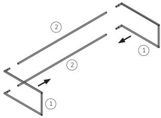
slide frame sides onto cross rails - no fixing required.
