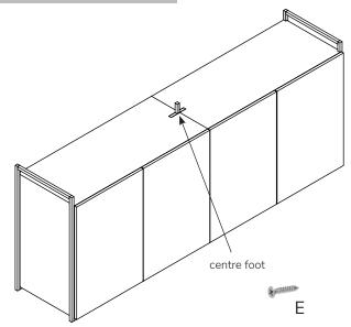
fix the centre foot to the underside of the carcasses with item  $\ensuremath{\mathsf{E}}$
