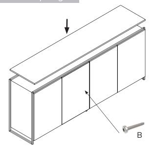
with the sideboard placed on its feet position the top and fix from inside with item B  $\times\,6$
