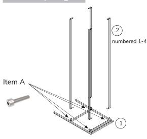
Place one of the side frames on the floor with the connections facing upwards. Then add the numbered horizontals into the matching number fixture on the side frame.
