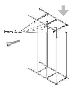
Once they are fixed in place position the other half of the extension side frame above and locate onto the four rails with the rest of ITEM A. You maybe need a mallet for this stage.
