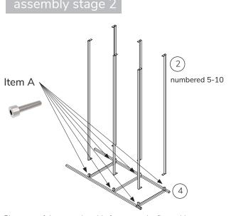
Place one of the extension side frames on the floor with the connections facing upwards. Then add the numbered horizontals into the matching number fixture on the side frame.
