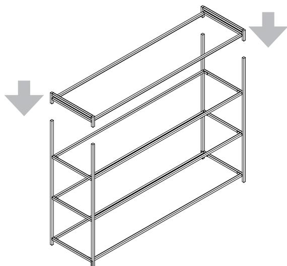
Position top frame over extension frame and slide into place
