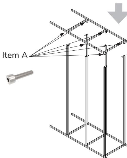
Once they are fixed in place position the other half of the extension side frame above and locate onto the four rails with the rest of ITEM A. You maybe need a mallet for this stage.
