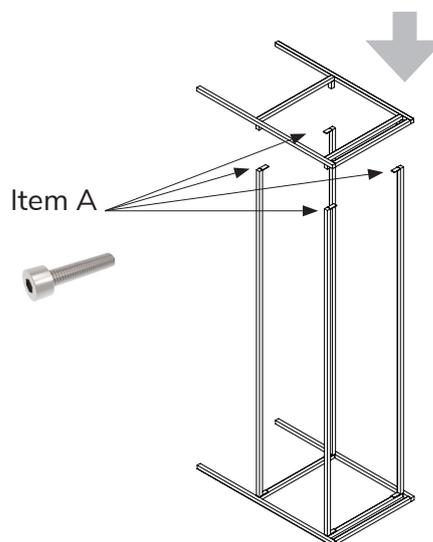
Once they are fixed in place position the other half of the side frame above and locate onto the four rails with the rest of ITEM A. You maybe need a mallet for this stage.
