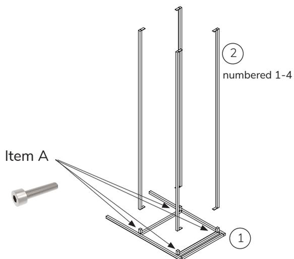
Place one of the side frames on the floor with the connections facing upwards. Then add the numbered horizontals into the matching number fixture on the side frame.
