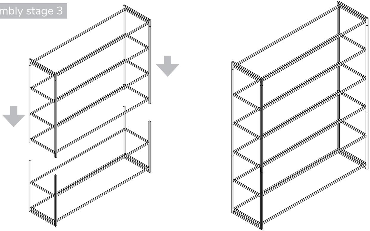
Position the extension frame and slot into the top of the base frame
