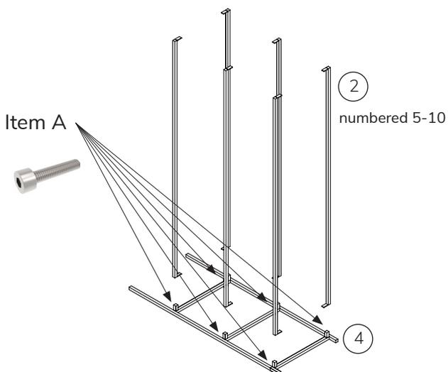
Place one of the extension side frames on the floor with the connections facing upwards. Then add the numbered horizontals into the matching number fixture on the side frame.
