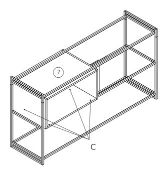
Position and fix cabinet from underneath centre rails lower and centre rails with screw C.
