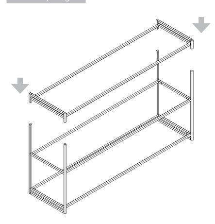
Position top frame over extension frame and slide into place.
