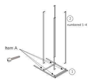
Place one of the side frames on the floor with the connections facing upwards. Then add the numbered horizontals into the matching number fixture on the side frame.
