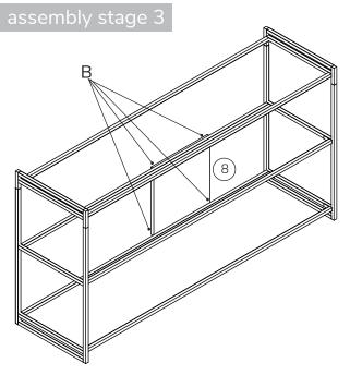
Position and fix panel to the back of the lower and centre rails with screw B.
