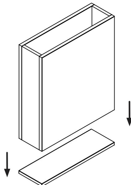
Gently press the back panel from inside the carcass to release.
