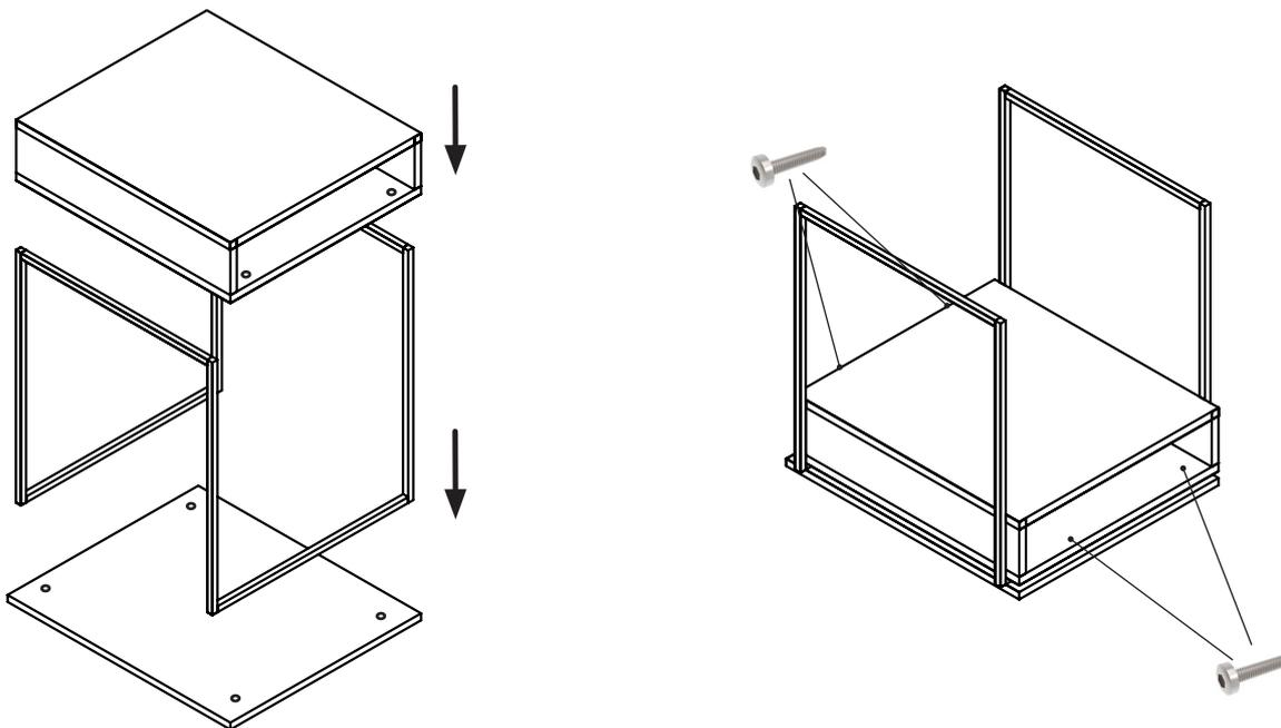
Position the frame upside down on the top and lower the carcass into place,
