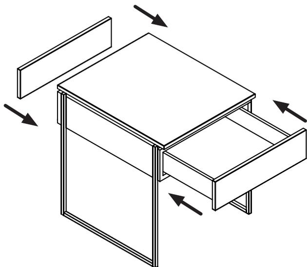
Press the back panel into its original position and securely engage the drawer back onto its runners
