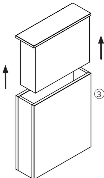
Remove drawer by pressing (in opposite directions) the small plastic lever on each runner.
