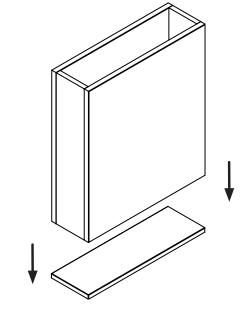
Gently press the back panel from inside the carcass to release.
