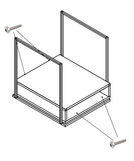
Secure the top and carcass to the frame using the bolts provided.
