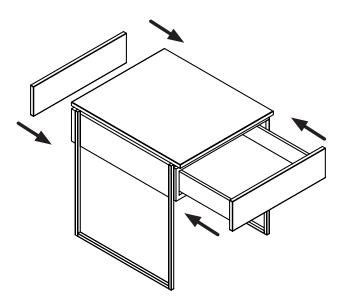
Press the back panel into its original position and securely engage the drawer back onto its runners
